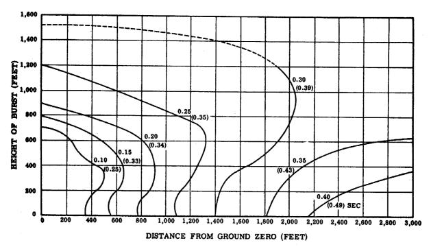
Figure 3.69. Positive phase duration on the ground of overpressure and dynamic pressure (in parentheses) for 1-kiloton burst.
