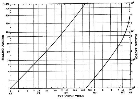
Figure 8.27b. Scaling factor for initial gamma-radiation dose.
