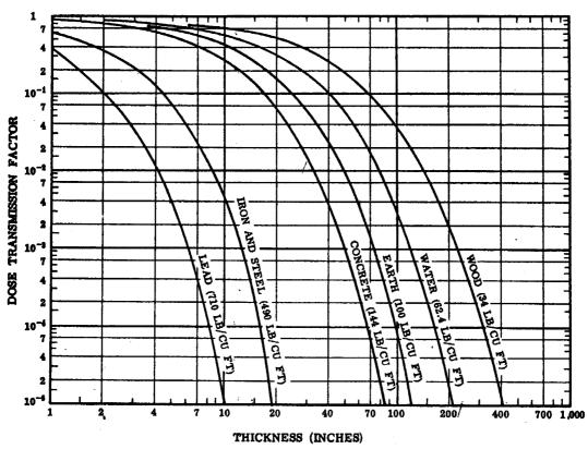
Figure 8.38. Dose transmission factors for initial gamma radiations of various materials as function of thickness.
