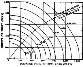
Figure 3.70a. Arrival times on the ground of blast wave for 1-kiloton burst (early times).
