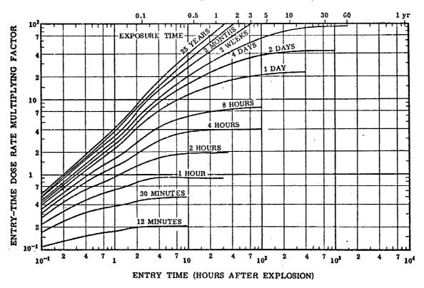
Figure 9.27. Total radiation dose from early fallout based on dose rate at time of entry.
