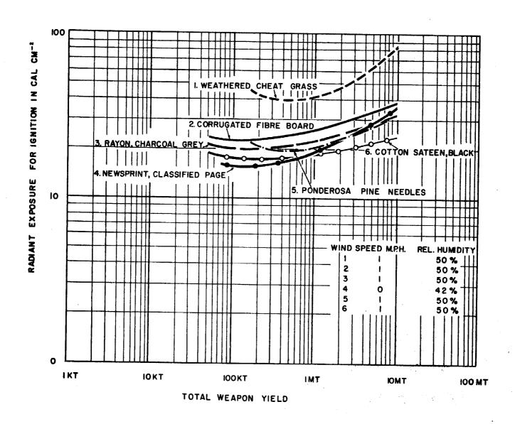
FIG.7.16.2 RADIANT EXPOSURES TO IGNITE VARIOUS MATERIALS AS A FUNCTION OF TOTAL WEAPON YIELD, TAKEN FROM TECHNICAL OBJECTIVE AW-7" by J. BRACCIAVENTI & F. DEBOLD, JULY 1960.
